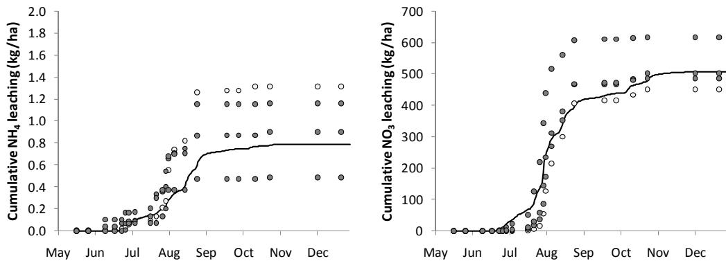
**Figure 2. Measured (points) and simulated (lines) values of cumulative N leaching as NH<sub>4</sub> or NO<sub>3</sub>.**
